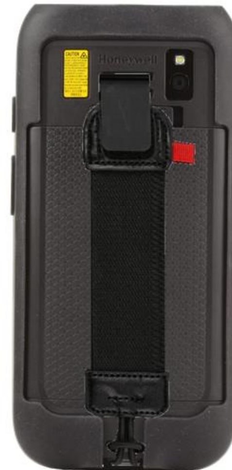
Rear View - Hand strap Installed
