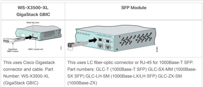
GBIC and SFP support depends on the platform and software version. Refer to these documents for GigabitEthernet system requirements, as well as GBIC system requirements, Coarse Wave Division Multiplexer (CWDM) GBIC, Gigastack GBIC, and SFP system requirements:
